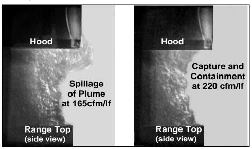
Figure 2. Schlieren images at different exhaust rates per linear foot (If).
