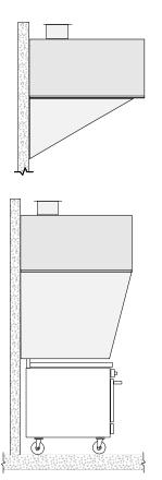
Figure 12. Illustration of partial and full side panels.
