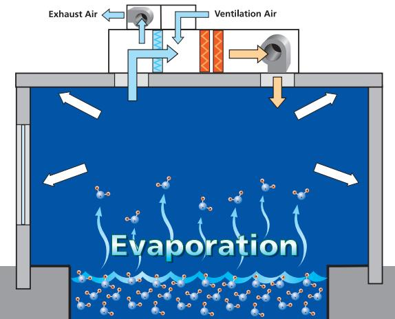
Figure 3 - Refrigeration-Based Dehumidification System
